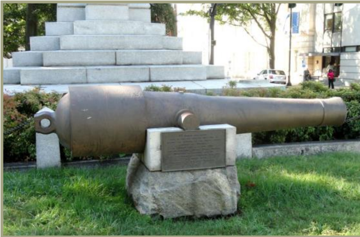
A 32-pounder Naval Cannon located on the grounds of the North Carolina State Capitol. Cast in 1848, captured at Norfolk in 1861, and converted to a 6 inch rifle for use at Fort Caswell. (Photo courtesy of Daderot via Wikimedia Commons)
