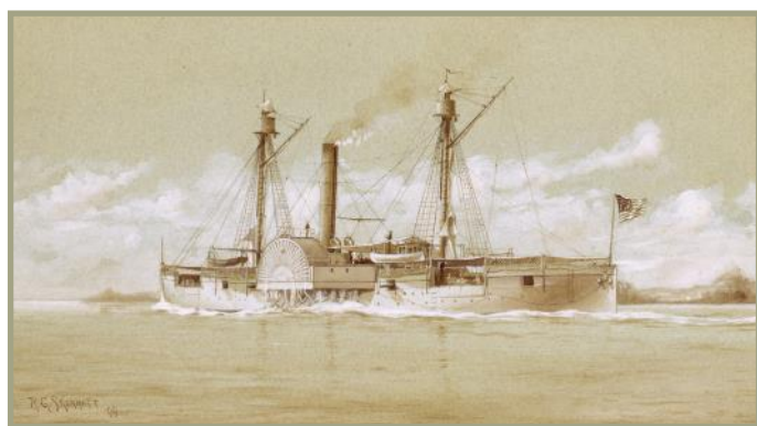
USS Agawam, a double-ender—a ship that had a rudder at each end to facilitate movement in narrow waters.
